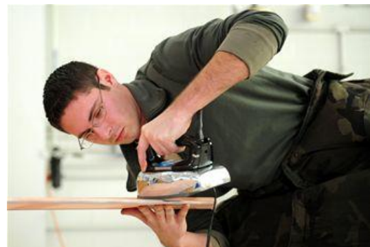
U.S. Air Force Airman 1st Class Christopher Morrison, 94th Aircraft Maintenance Unit avionics specialist, applies the skin to a wing of the Nieuport 28 replica at Langley Air Force Base, Va., Jan. 17, 2012. The French-made Nieuport was among one of the first aircraft to be taken into battle by the 94th Fighter Squadron at Langley AFB. (U.S. Air Force photo by Airman 1st Class Kayla Newman/Released)
